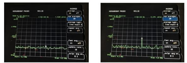
Figure 7. Received sum frequency component in the absence of a bubble in the interaction region. Received sum frequency component in the presence of a bubble in the interaction region. The transmitted primary frequency components are 2.21 and 2.20 MHz. The scattered sum frequency component is at  $f_+ = f_1 + f_2 = 4.41$  MHz. Horiz. Scale is 2 kHz/Div. Vert. scale is 3 micro Vrms/Div.
