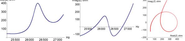
Figure 4. Left to Right: The real part and imaginary part of the electrical impedance Z of the cylindrical shell transducer vs. frequency; the circular impedance plot of the transducer (real {Z} vs. imaginary {Z}).
