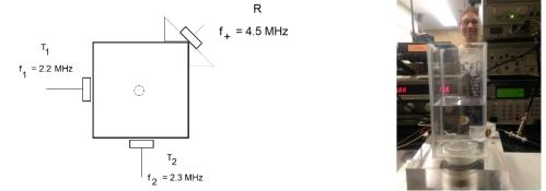
Figure 1. Left to right: Top view of non-linear scattering setup of crossed ultrasonic beams in the presence of a levitated air bubble in water; combined acoustic cell levitation apparatus with crossed beam transmitting and receiving transducers, and co-author KAH.
