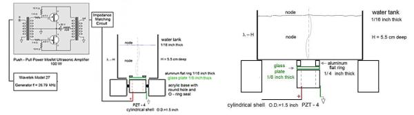
Figure 2. Supporting electronics with levitation cell #1 (tank base 5.7 x 5.7 cm<sup>2</sup>) and cell #2 (12.5 x 12. cm<sup>2</sup>).
